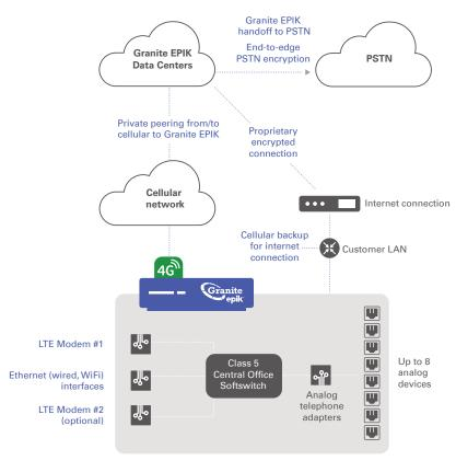
Choice of cellular, wired Ethernet, WiFi or PRI as primary network connectivity, with automatic failover to any option.
